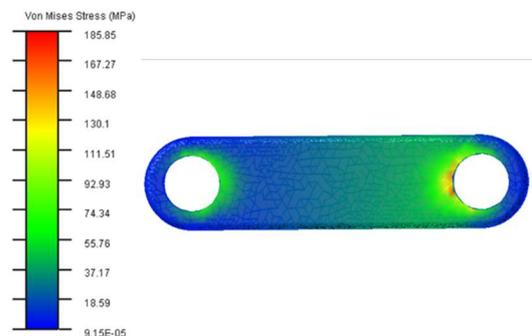
*Fig. 6 Stress distribution of front toggle lever*
