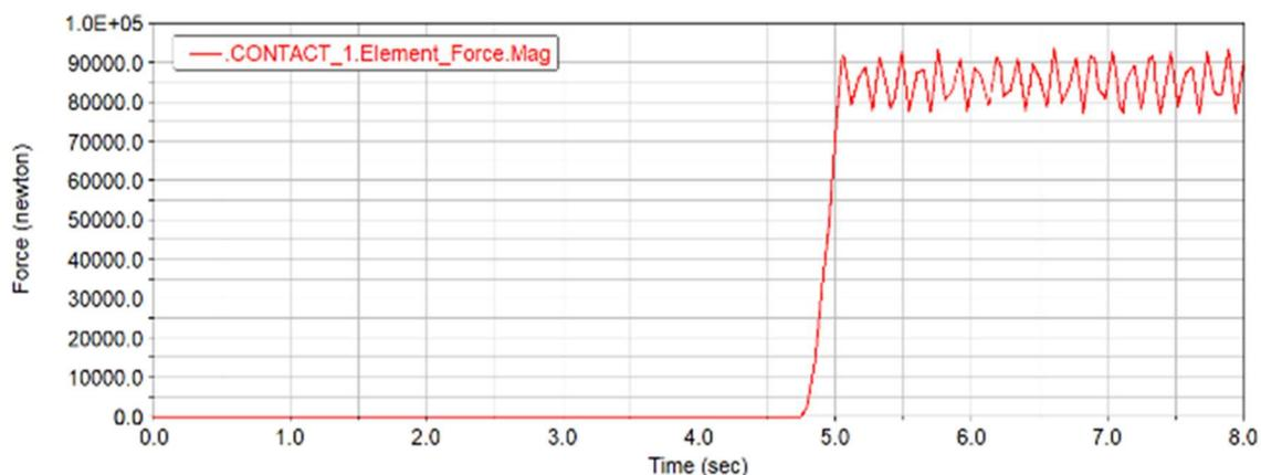
Fig. 3 The clamping force vs. time
