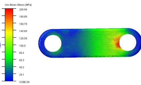
*Fig. 8 Stress distribution of side rear toggle lever*
