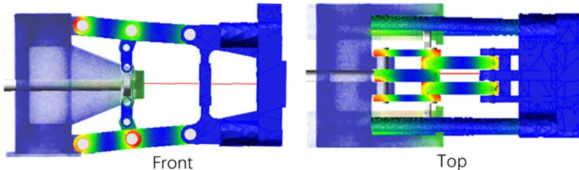
*Fig. 4 The stress distribution of the toggle mechanism*
