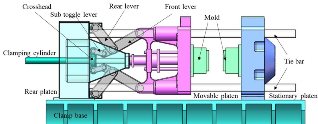
*Fig. 1 the mechanical system of the injection molding machine*
