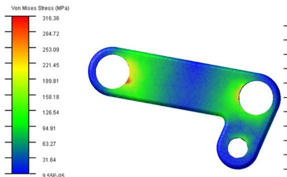
*Fig. 7 Stress distribution of mid rear toggle lever*
