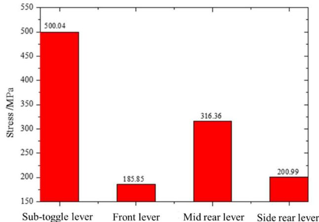
*Fig. 9 The maximum stress on each lever*
