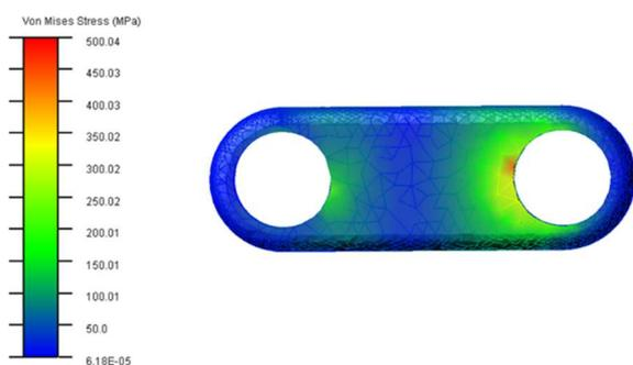
*Fig. 5 Stress distribution of the sub toggle lever*
